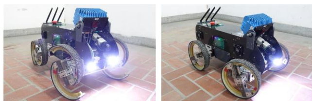
Fig. 1 The leg-wheel transformable robot TurboQuad-V .
