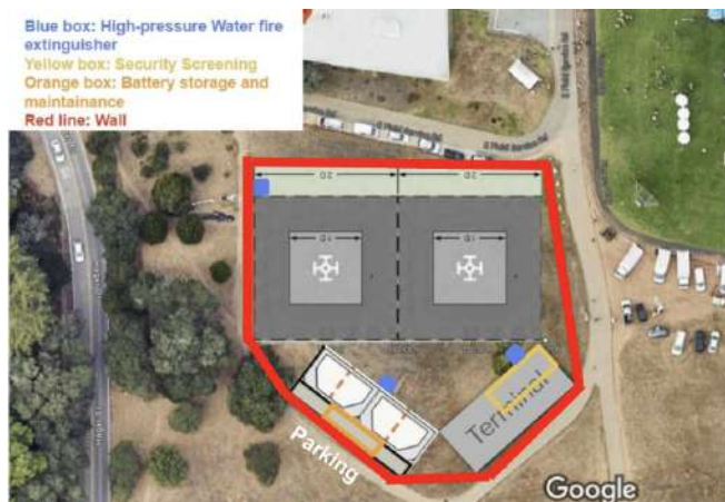
Figure 9. UC Santa Cruz vertiport location layout from the aerial view, showing two constructed vertiports and connected infrastructure.
