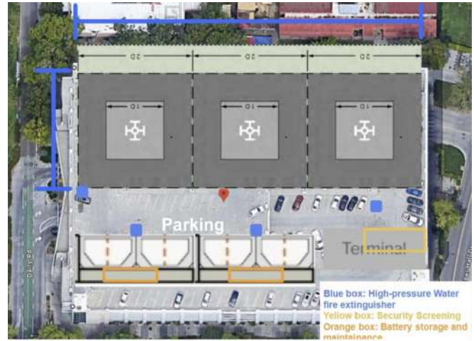
Figure 7. UC Davis vertiport location layout from the aerial view, showing three constructed vertiports and connected infrastructure.
