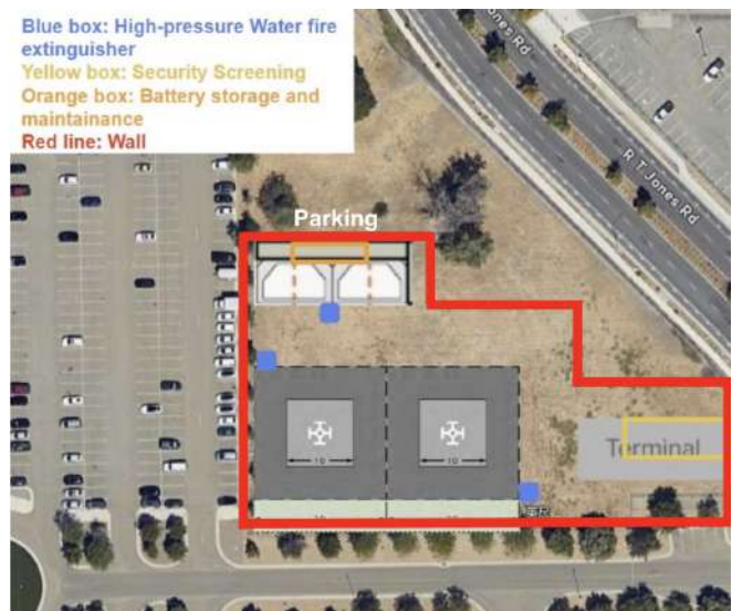
Figure 10. NASA Ames vertiport location layout from the aerial view, showing two constructed vertiports and connected infrastructure.
