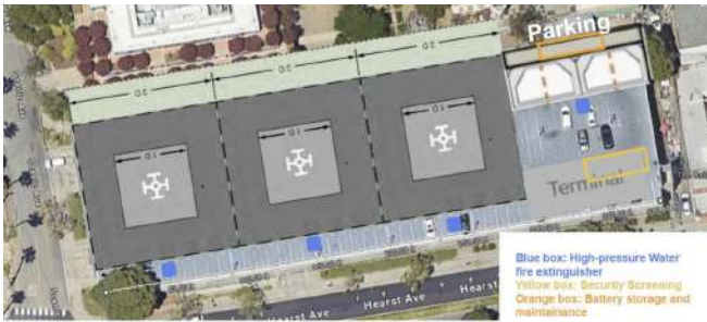
Figure 6. UC Berkeley vertiport location layout from the aerial view, showing three constructed vertiports and connected infrastructure for parking and refueling.
