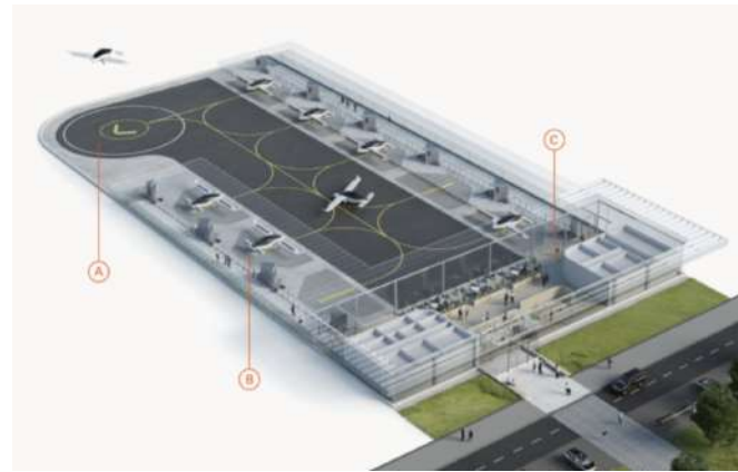
Figure 4. Example vertiport layout. A) TLOF, B) Parking stations, and C) Terminal
