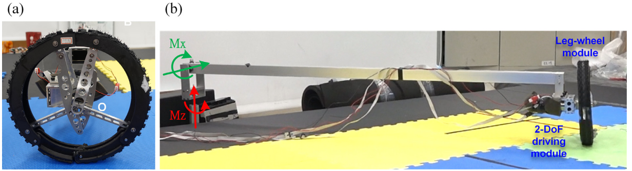
Fig. 14. The leg-wheel module: (a) side view of the module and (b) the module with a boom in experiments.
